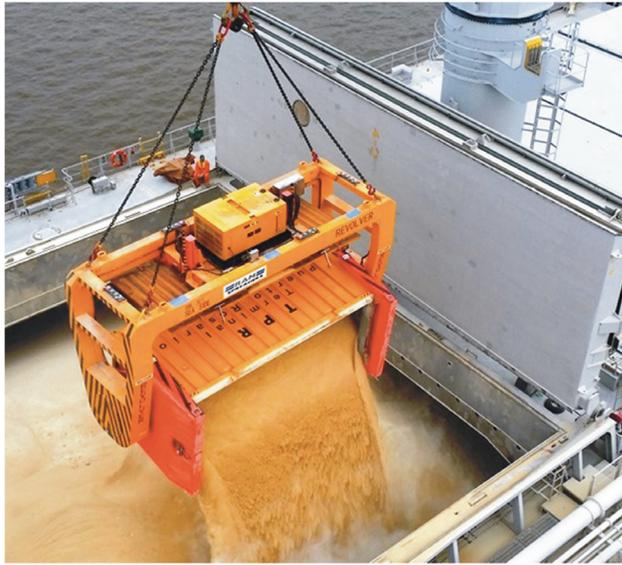
RAM Revolver on ship's crane lifts lid and tips grain into ship's hold.
