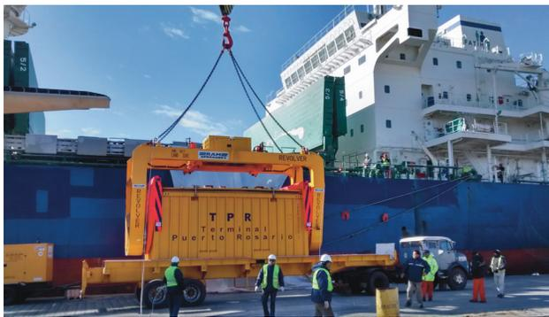
RAM Revolver lifting container directly from truck for unloading into a ship's hold.
