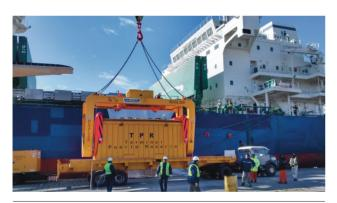
RAM Revolver lifting container directly from truck for unloading into a ship's hold.
