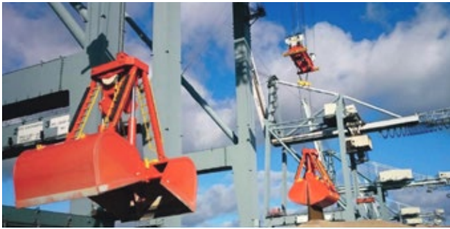
Adapted STS container cranes in Aarhus, handling building materials, which can quickly be returned to container handling.
