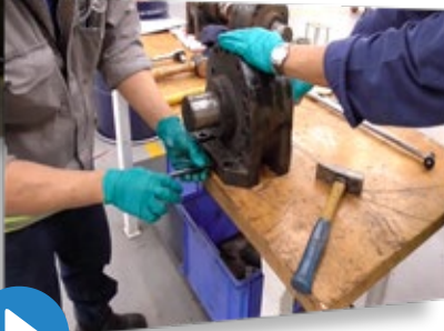
▶ How to replace the seals on a hydraulic actuator normally found on a RAM Spreaders hydraulic spreader
