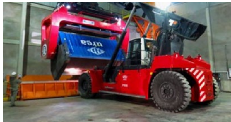
The SMAG grab unloads the ship into container and the RAM Revolver unloads the bulk at destination. Simple and no dust!
