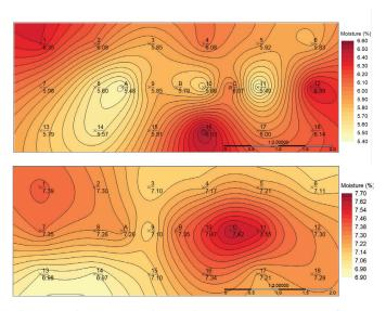
Above: Sampling stage two showing the average moisture content for samples (above). Sampling stage three, average moisture content for samples, both obtained from a 21-point sampling template, (shown in image 2) representing the entire depth of the material (scale in metres)
