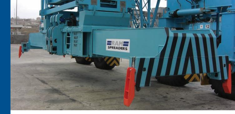
The RAM 3900 series All Electric Twinlift CenterSpread® has been developed to provide productive, safe and cost-effective container handling for both ship-to-shore cranes and yard stacking cranes.
