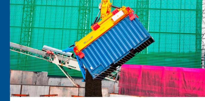
The RAM Tilting Spreader Model 2780 has been designed for use on Mobile Harbour Cranes and jib cranes to handle standard ISO 20ft hatch door containers for cost effective handling of bulk commodities. The spreader also has the capacity to act as a standard 20ft fixed spreader for handling conventional 20ft ISO containers.
