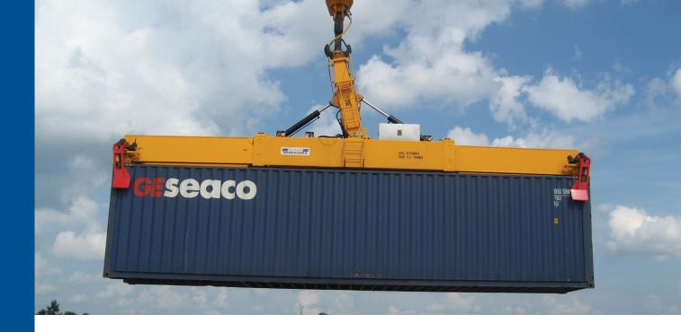
The RAM 2700 series of Electro-Hydraulic Telescopic Spreaders including twinlift has been developed to provide productive, safe and cost-effective container handling for mobile harbour and jib cranes. Six models provide a wide choice of capacities from 35 to 65 tonnes designed to handle single 20', 40' and 45' containers. 2740, 2750 and 2760 models also provide twinlift capability, designed to handle two 20' containers as well as the full range of single container lifts.
