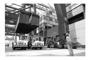
Figure 1 Dual Hoist STS Crane
