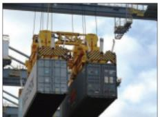
design. The smart headblock can transfer from Single to Tandem to Quad quickly and without the need for ground staff. This transformation is achieved in a docking station with an auto-electrical connector. The automated change-over from single to tandem mode for SingFlex is world's best design in tandem. It is performed by the crane operator and is achieved in less than 2 minutes.
