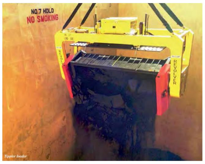
any product being poured into the corner casting thus, saving on any clean up requirements and crane down time. The internals of the containers are painted with special paints to stop corrosion. "The revolver is the only item required at an unloading facility and can be attached to any STS, ships or mobile harbor cranes or reach stacker. Lid lifter using the ISÖ patented lid lifter, the system is automatic and eliminates labor and product loss." adds Mr. Srikanth.
