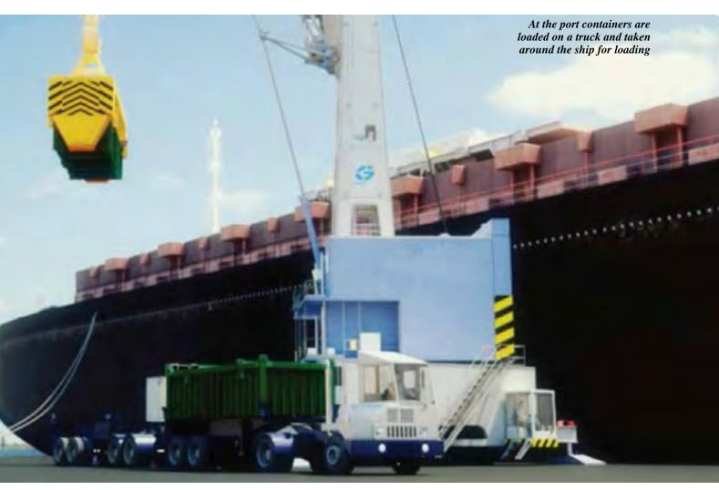
are loaded at the production facility, either by loading chutes or conveyor belts into the container roof hatches. Once loaded, the containers are sealed and the lid is not removed again until the bulk product is ready to be emptied. The containers are transported by road or railway wagon rakes to the loading ports, where the cargo is emptied into the vessels from the containers for further shipment."
