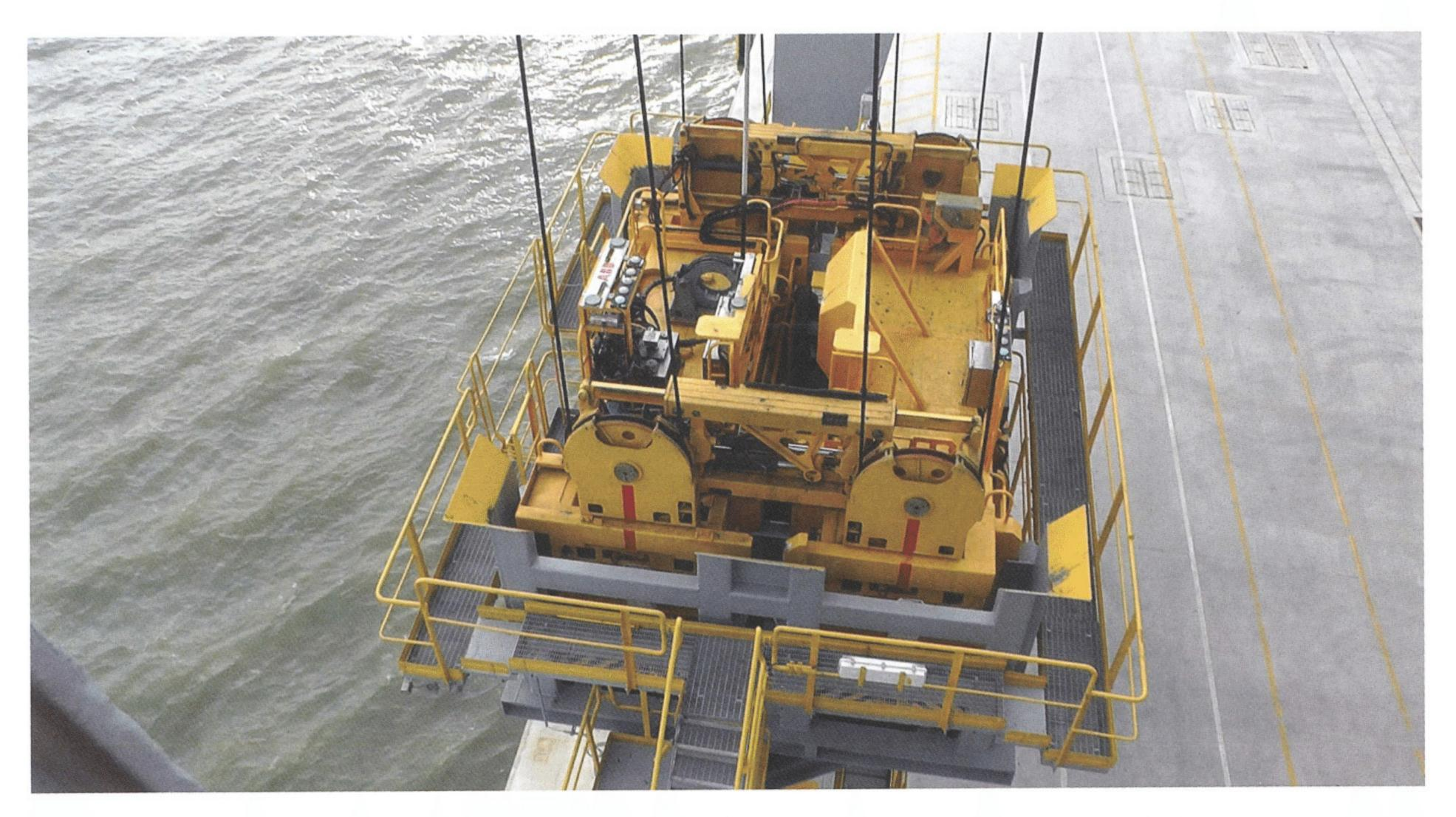
and uses a conventional crane design. It employs a "smart" headblock that can automatically switch from single to tandem mode, which allows two spreaders to be attached to a single hoist crane.
